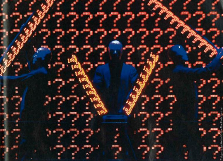
On the Vegas stage, destination displays include three LED walls plus "flyin" front and rear projection screens. To the left and right of the central LED screen, two "abstract" spiral LED screens are also used. Inputs to the Encore system include robotic cameras, live cameras, high-resolution graphics from Catalyst media servers, and digital playback from Doremi V1 videodisk recorders. Encore also controls the system's analog and digital routers.
