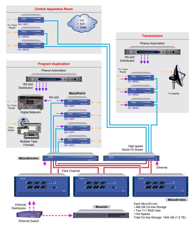
The Omneon system consists of two MEDIASERVERs, five DV/MPEG MEDIAPORTS, five SDI/SDTI MEDIAPORTS and three MEDIASTORES, each of which includes two 7+1 RAID sets and 498 GB of available storage. Total system capacity is 1.5 Terabytes. Each MEDIASERVER connects to each MEDIASTORE via three Fibre Channel loops for maximum bandwidth. All MEDIAPORTS connect to the MEDIASERVERs using high-speed serial I/O buses that each provide up to 400 Mbps of bandwidth.
